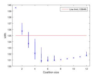
**Fig. 5.** Plot of the maximum hourly average power vs coalition size for Problem 2. The lines indicates the range of values, and crosses mark the mean for each coalition size.
