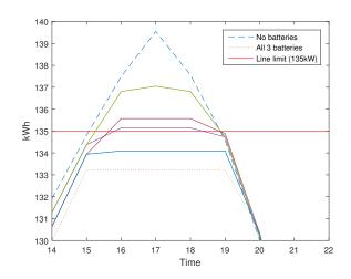
Fig. 3. Load profiles for optimal load relief by all six sub-coalitions in the copper-plate model, with the line limit indicated.
